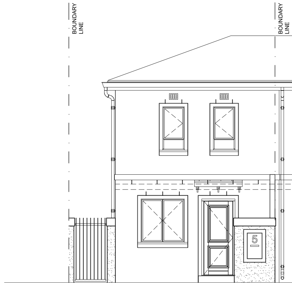
TYPICAL STREET ELEVATION
